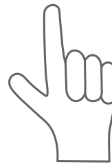
Beginning of rope reeling from the left side of the drum for the left-lay rope
